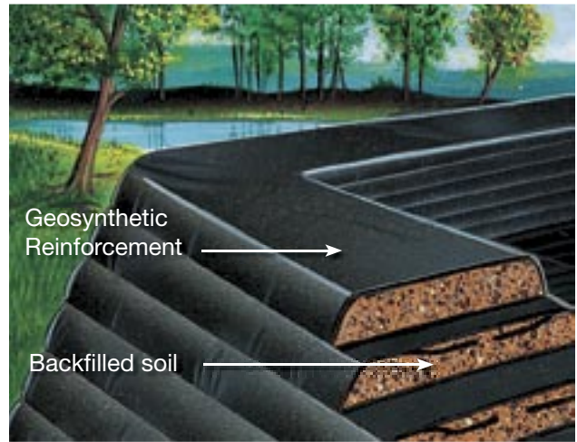
Internally reinforced earthwall
